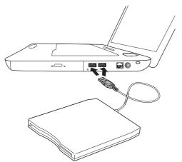
Figure 8-7 Connecting the USB floppy diskette drive
